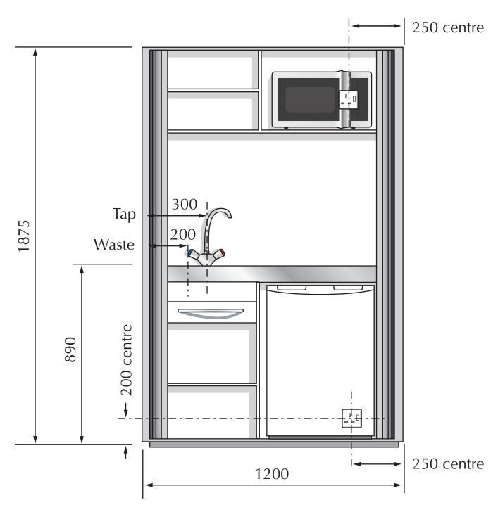
**Electrical Consumption** All appliances fitted with 13amp plugs with 1.2 metre flex
